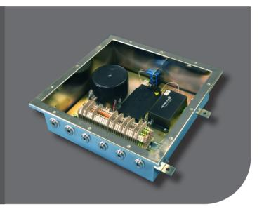
The Power Supply Unit and Media Converter has been designed for both toughness and durability as demanded for operation in the most adverse of environments. The 316L stainless steel enclosure combined with a unique design of the Ex eb mb product eliminates the need for an Ex d junction box.
