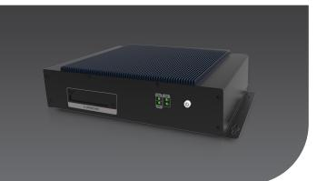
The latest evolution of Synectics' T-series Network Video Recorder (NVR), the T2000, brings IoT-ready functionality to the on-vehicle market and can support up to 16 full-HD digital cameras\*.
